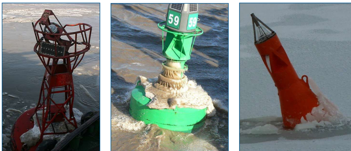
Figure 11 Effect of ice on buoys
